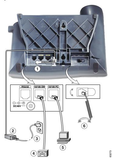
Figure 3-2 Cisco IP Phone Model 7910 Cable Connections
